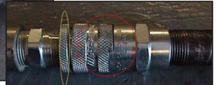
Lock-Down screw is highlighted in yellow. Highlighted in red are the two components that twist lock and snap together.
